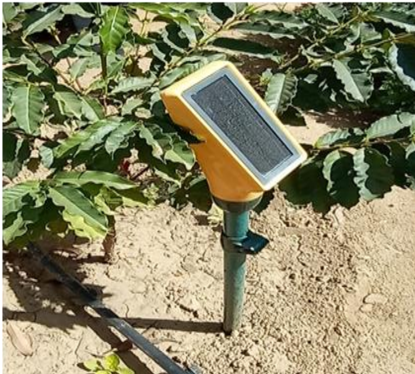
Figure 24: A solar powered soil water moisture meter Al Dayer, Jazan
